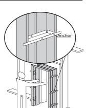
**5.** Place temporary wooden spreaders between the jambs of the frame. The spreaders must be square, at least 1" thick with clearance notches at each end for the frame stops/soffits, and cut to the exact width of the opening
