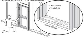
Level header and shim up from floor as
