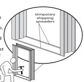
Verify rough opening is correct size and framing is plumb and square.
